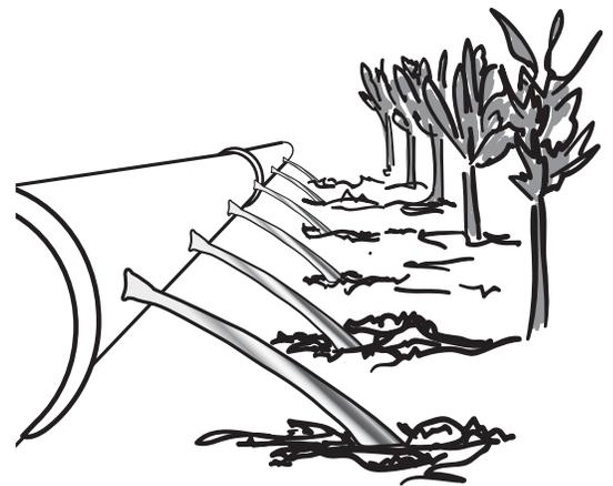
If you're already using gated pipe, you may be able to save additional energy by installing a surge valve. Surge valves automatically alternate the water from one set of furrows or border strips to another. This method causes the water stream to advance much faster. Deep percolation at the upper end of the field is reduced and water penetration at the lower end is increased, resulting in more even water distribution.
